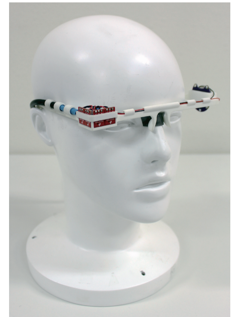
3D-printed wearable sound localization prototype, placed on the dummy head. It contains four INMP401 MEMS microphones separated by 20 mm, powered by a CR2032 battery. The processing unit is not included in this early version.
